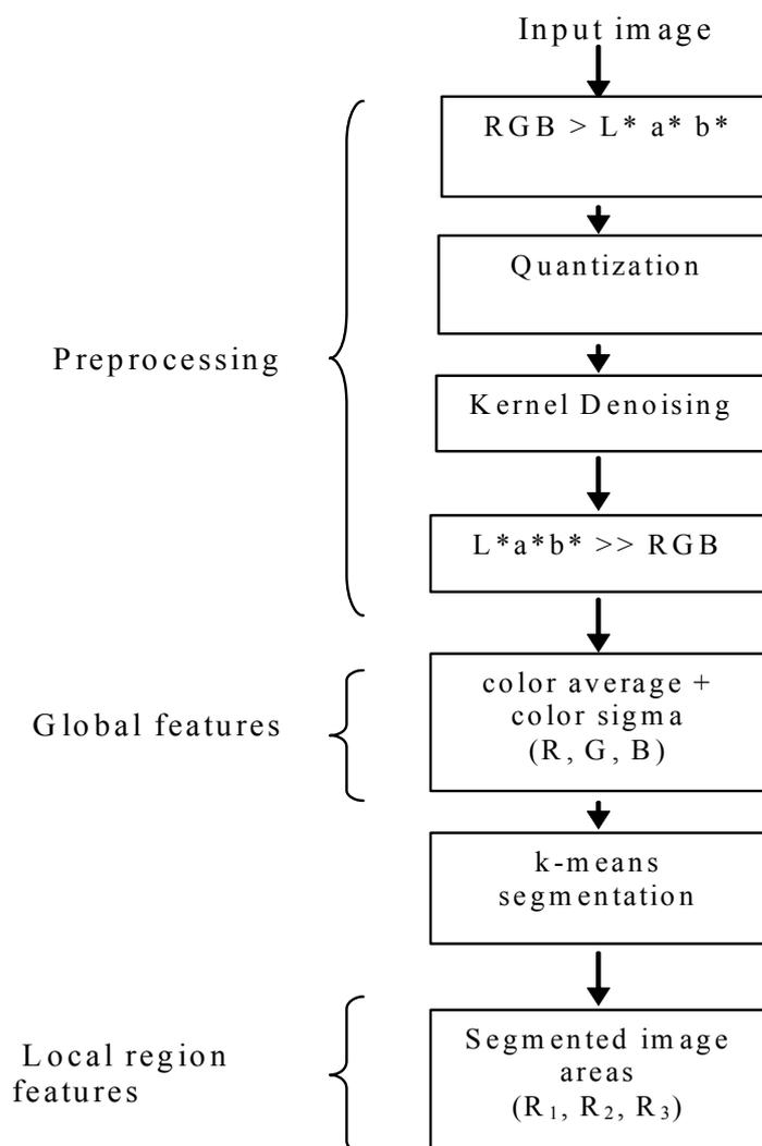
**Figure 2** Block diagram for the proposed methodology.
